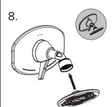
Ensure the rubber seal for shower head is intact then fit and tighten the shower head to the screw cap and stem. Check operation. Handle should swing from right to left from OFF to HOT. Total movement is about 130°.
