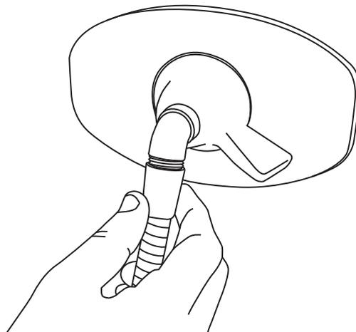
3. **For Mains Pressure, fit flow restrictor into the handpiece first.**
