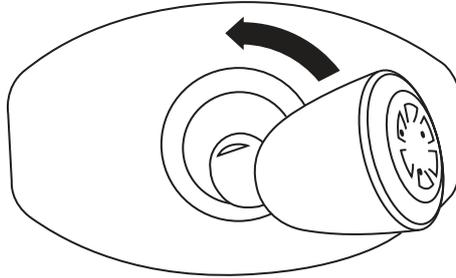
1. Remove the shower head from the existing Feltonmix wallset by gripping the shower head stem and turning it anti-clockwise.
